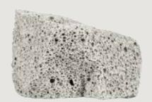
For perimeter insulation with high load requirements, such as commercial and industrial buildings, but also for light-construction trafficable areas, squares, and streets. Very good long-term settlement behaviour. Very high stability.
