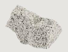
For lightweight fillings with the highest load requirements and dynamic loads, such as roads and airstrips. Extremely high stability, extraordinary long-term settlement behaviour.
